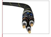
Power Cable: For transmitting power from the generator mounted in the nacelle of the wind tower to base station. Flexible cables made of special elastomeric compounds to meet torsional stresses exerted to rotation of the nacelle in relation to wind direction.
